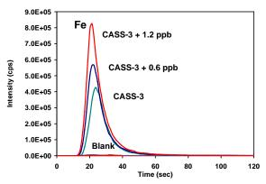
blanks and eliminates pump noise. Smooth elution profiles (3 point moving average) illustrate the high signal to blank ratio and standard additions to CASS-3.
