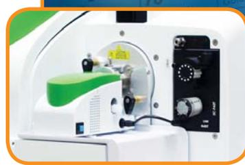
Integrated PC<sup>3</sup> FAST DXi for the NexION 300 showing 4 channel precision peripump, FAST valve and PC<sup>3</sup> Peltier cooler.
