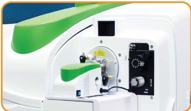
The PC<sup>3</sup> is a small, robust Peltier cooled cyclonic spray chamber. The PC<sup>3</sup> offers the advantages of low memory effects, constant temperature, fast rinse-out and high sample transport efficiency. The cooled outer walls of the PC<sup>3</sup> spray chamber enhance long-term signal stability, reduce polyatomic interferences such as oxides and reduce solvent loading when volatile organic solvents are analyzed.
