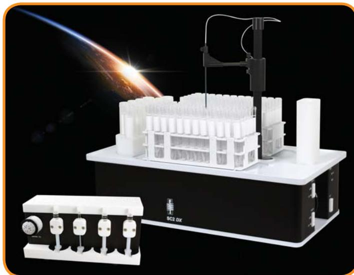
Samples are rapidly (0.5 mL/sec) and reproducibly vacuum loaded into a sample loop. Inside the valve, sample is mixed with the diluent and internal standard. The system delivers the diluted and mixed sample to the nebulizer with final dilutions ranging between 1x and 400x.
