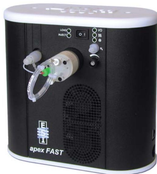
apex FAST with injection valve adjacent to nebulizer ES-43FH-21-52
