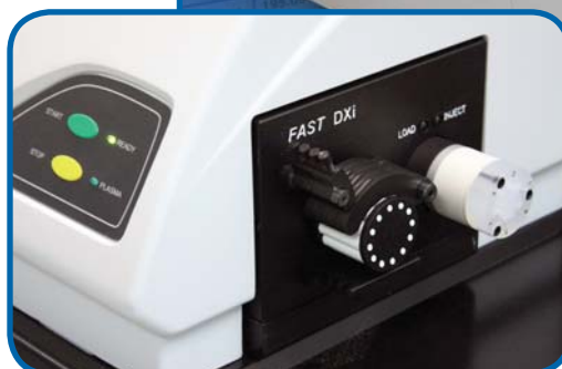
FAST DXi integrated into PE ELAN showing 4 channel precision peripump and FAST valve.
