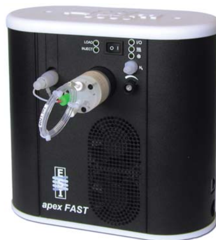
apex FAST with injection valve adjacent to nebulizer ES-43FH-21-94
