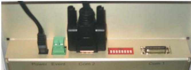
**Figure 6: AS-93+ Connections & Switch.**
