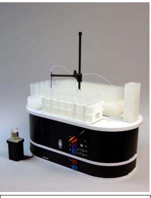
The FAST system integrated to the SC-2 autosampler includes control of an inert injection valve for sample injection or chromatography applications.
