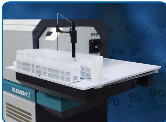
SC-E4 DXS integrated on the Thermo **ELEMENT 2** ICPMS with integrated MP<sup>2</sup> micro peristaltic pump
