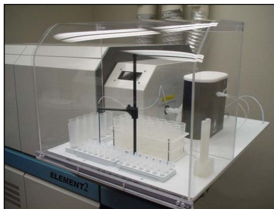
SC-E2 autosampler with clean enclosure attached
