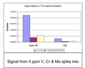
Sensitivity was increased 7 - 8 fold for the range of elements when compared to the standard introduction system. The Apex HF also consumes less than half the sample of the SIS.
