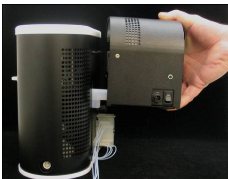
Membrane desolvation modules attach quickly and easily to the Apex outlet
