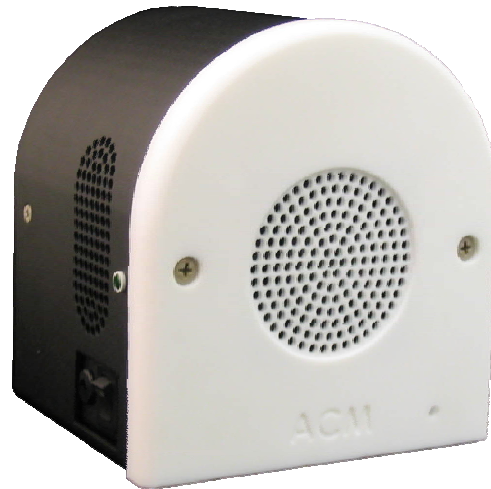
ACM Module cooled membrane desolvation unit
