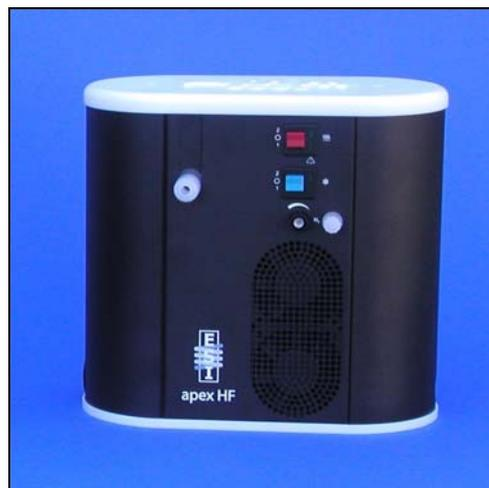
Apex HF high sensitivity, HF resistant sample inlet system
