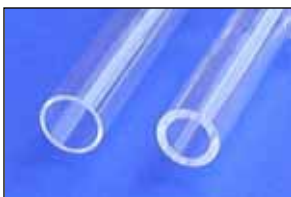
CD-type torch (left) vs. Precision quartz torch
