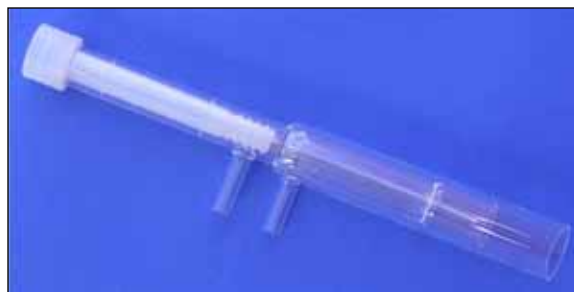
Quartz injector with 12/5 ball joint connector
